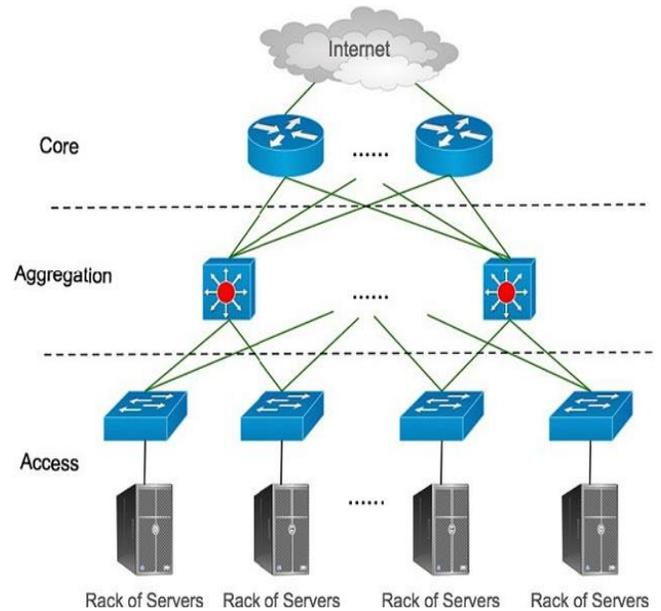
Fig 3: Cloud Data Center Architecture
