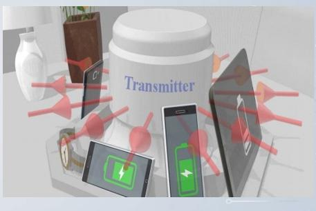
This issue can be solved by using several transmitter coils connected to several power sources for creating a strong charging field. However, this approach increases the complexity of the transmitter. While feedback can properly orient the charging field, the control systems themselves are also complicated and expensive.
