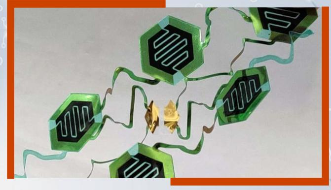
These devices consist of flat wires, called interconnects, as well as sensors, power sources and antennas to communicate data to smartphone apps or other receivers. To maintain full functionality, they must stretch, flex and twist with the skin and organs they are mounted on—without generating strains that would compromise their circuitry.
