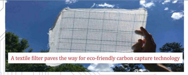
The researchers chose a piece of cotton cloth, known for its versatile properties, and a naturally-occurring enzyme called carbonic anhydrase to create the fabric, whose special property is simply removing carbon dioxide molecules from a gas mixture.
