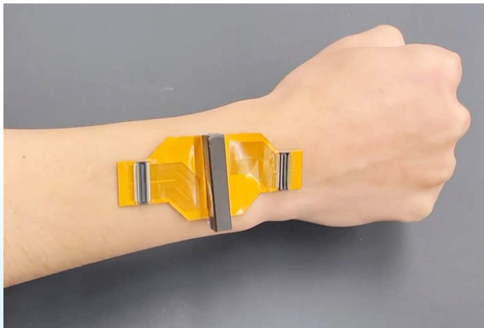
MIT's ultrasound sticker enables continuous monitoring of organ stiffness, revolutionizing the early detection of diseases such as liver and kidney failure.
