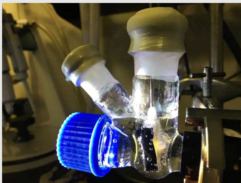
A photoreactor with an artificial leaf working under solar irradiation
