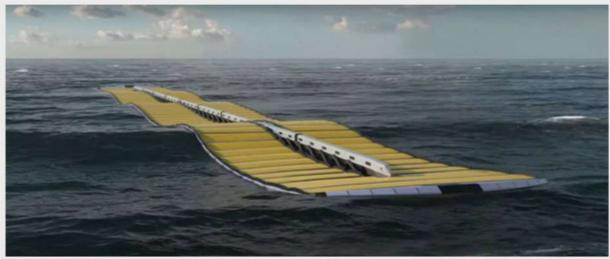
A unique spine-like floating device designed by a startup based in Cyprus promises to harness the energy of the waves and convert it into electricity.
