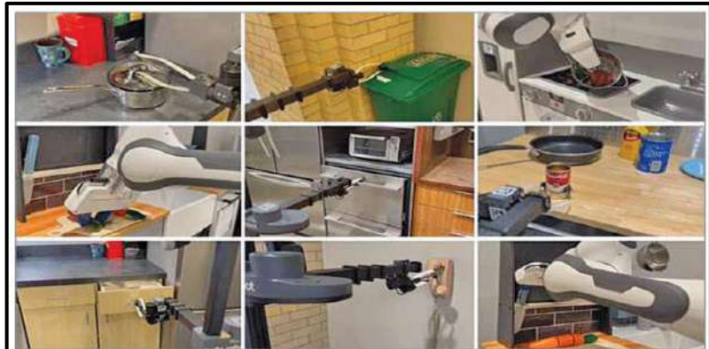
A team from Carnegie Mellon University's Robotics Institute used affordances to teach robots how to interact with objects (Credit: Carnegie Mellon University)
