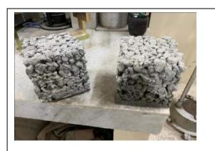
Fig. 1. Cubes of Pervious Concrete
